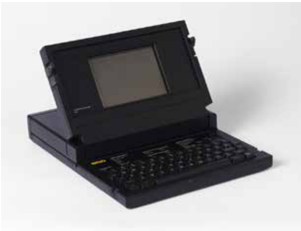
GRiD Compass Laptop Computer Prototype, 1981. Designed by Bill Moggridge (English, 1943–2012). Manufactured by GRiD Systems Corporation (USA). Die-cast magnesium, injection-molded plastic. Collection Cooper Hewitt, Smithsonian Design Museum, gift of Bill Moggridge, 2010-22-1. Photography: Matt Flynn.
