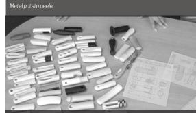
OXO and Smart Design developed many prototypes to better understand the effects of different handle shapes and materials on the peeler's design
