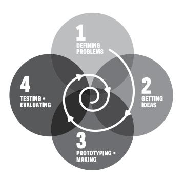
The spiral diagram shown here represents one way to look at the design process. Design thinking doesn't follow a straight linear path. The phases of the process often overlap, occurring simultaneously and circling back on themselves.
